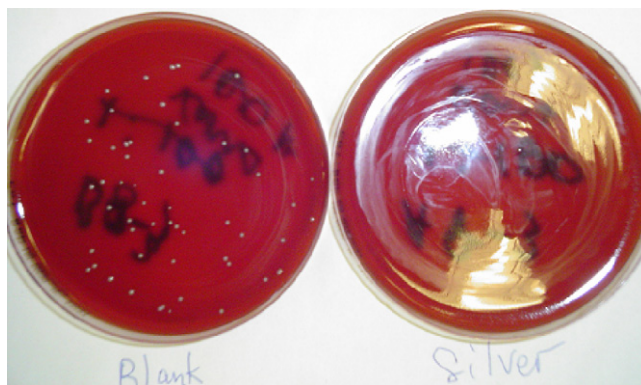
Fig. 6. Agar plates after incubation with solutions of S. aureus . The reference sample (left) clearly shows colonies while the sample which was in contact with a nc-Ag/SiCN nanocomposite is free of any bacteria colonies (right).
